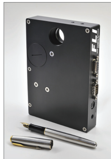
The HS-625 changes to the adjacent filter in as little as 23 milliseconds.
