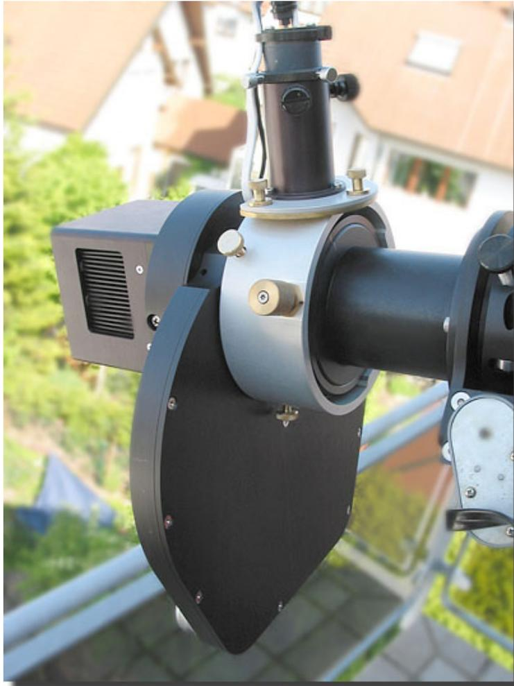
Camera and filter wheel with self-built off-axis-guider
