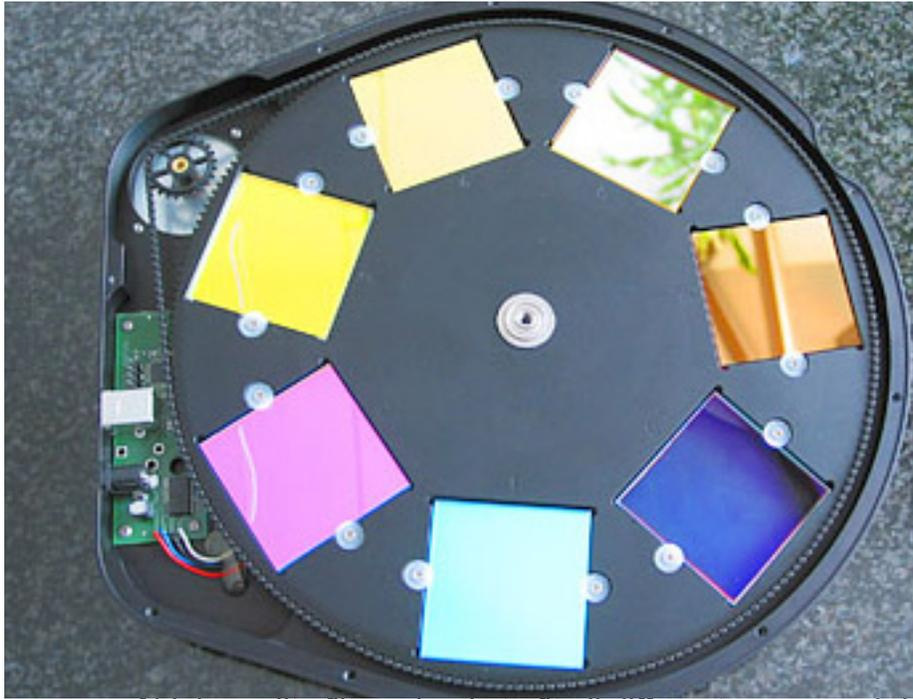
FLI offers a wide range of high quality filter wheels to fit all different cameras. I decided to purchase a CFW-5-7. This milled filter wheel can hold 7 unframed 50 mm x 50 mm filters. I use filters from the Baader-Planetarium company: Luminance, red, green, blue, H-alpha (7 nm), OIII (8.5 nm) and SII (8 nm)
