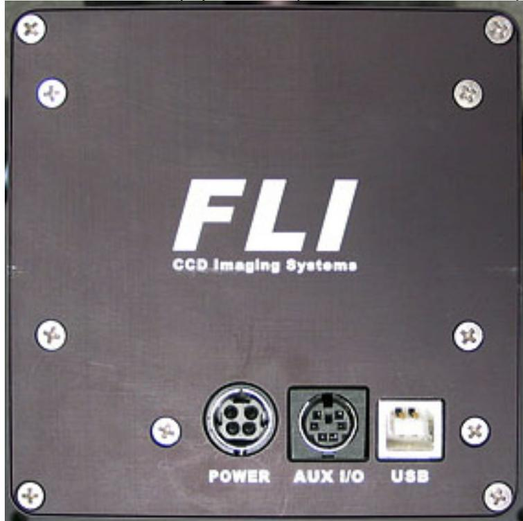
Connections from left to right: Voltage supply 12V, external trigger, USB 2.0-data interface
